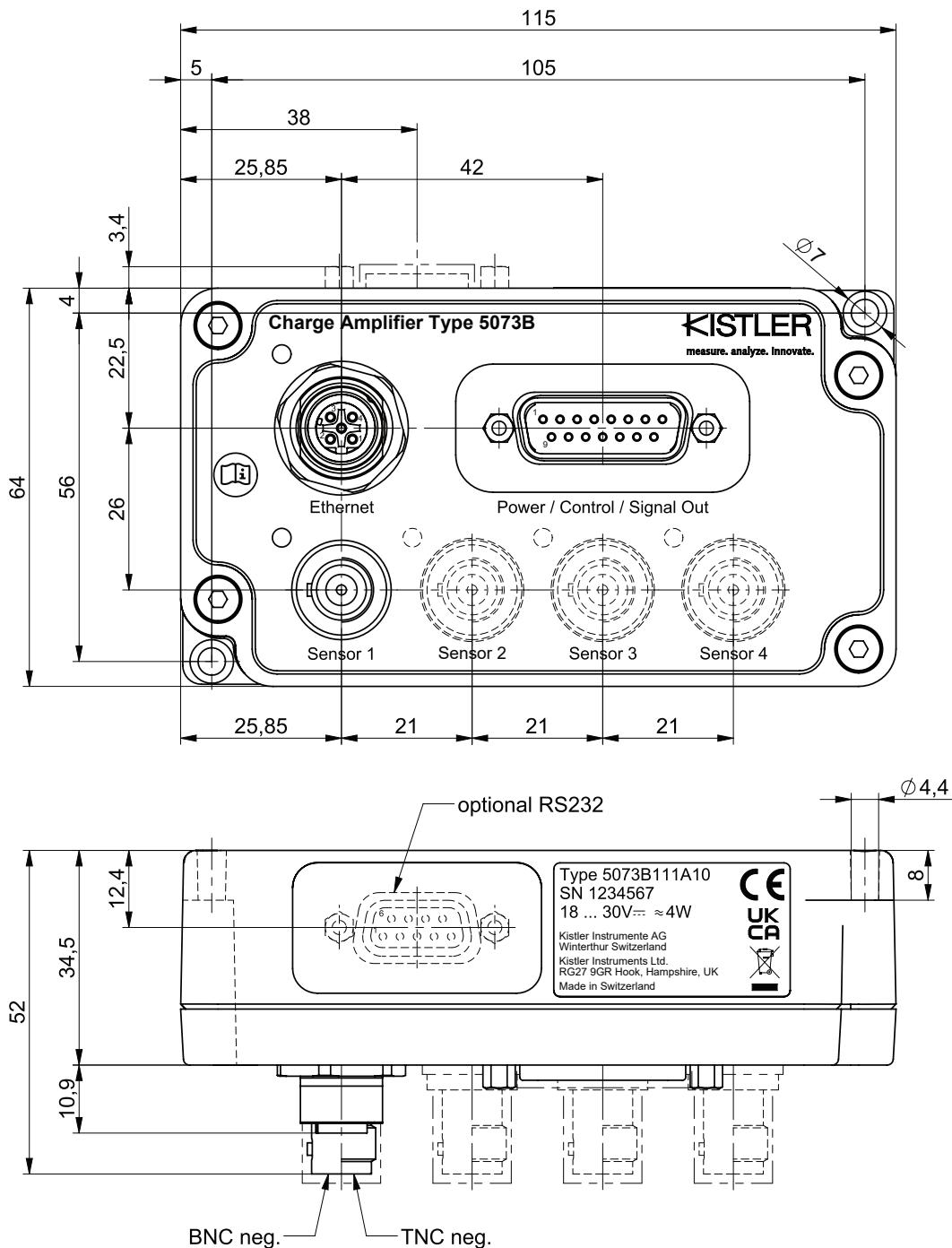
ICAM B – Industrial Charge Amplifier for Multi-purpose with Ethernet, Type 5073B...
